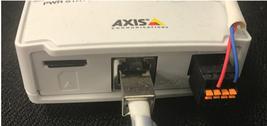
Figure 1: Door sensor wiring for AXIS 2014E
